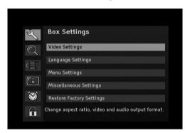
By using the **arrow button** ▲ or ▼, highlight the desired option and press the OK button in order to call it up.
